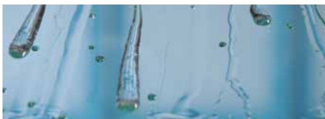
Glass treated with RAVAK AntiCalc® - water is repelled and runs down the glass.
